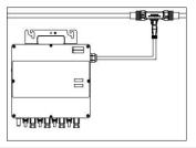
NOTE: AC connector interface as follows, from left to right PE, N, L3, L2, L1.
