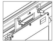
Step 4. Connect the APsystems Microinverter cables to the AC bus cable.
