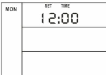
The last digit in the time flashes. Enter the minute (unit) setting and press the “MODE” button. The digit setting is defined and the minute (tens) digit starts to flash. Enter the minute (tens) setting and press the “MODE” button. The first digit of the hour display starts to flash. Enter the hour and weekday settings in the same way as the minutes setting.
